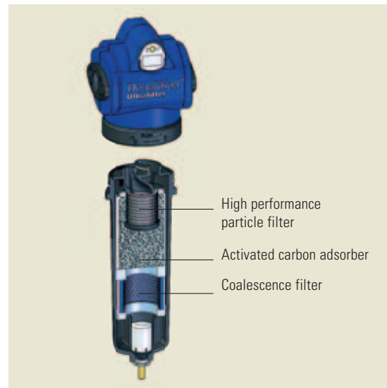
Cross-section of an Ultra-Filter with DF-T element
